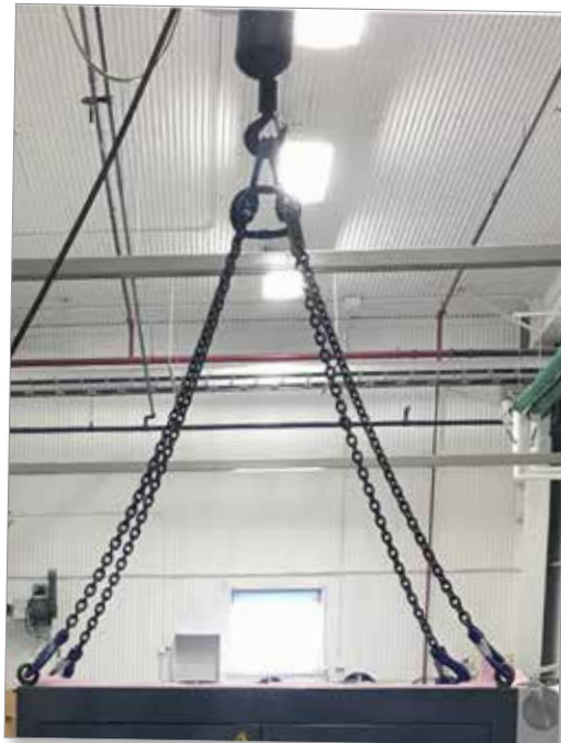
Figure 3-11 Attach slings to all four eyebolts
