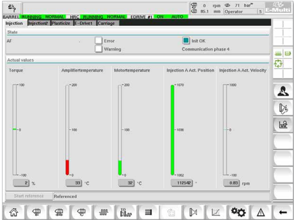
Figure 7-33 Drive monitor screen
