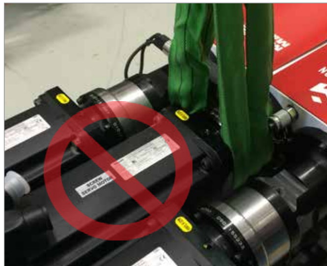
Figure 3-12 Do not use the motor as a lifting point
