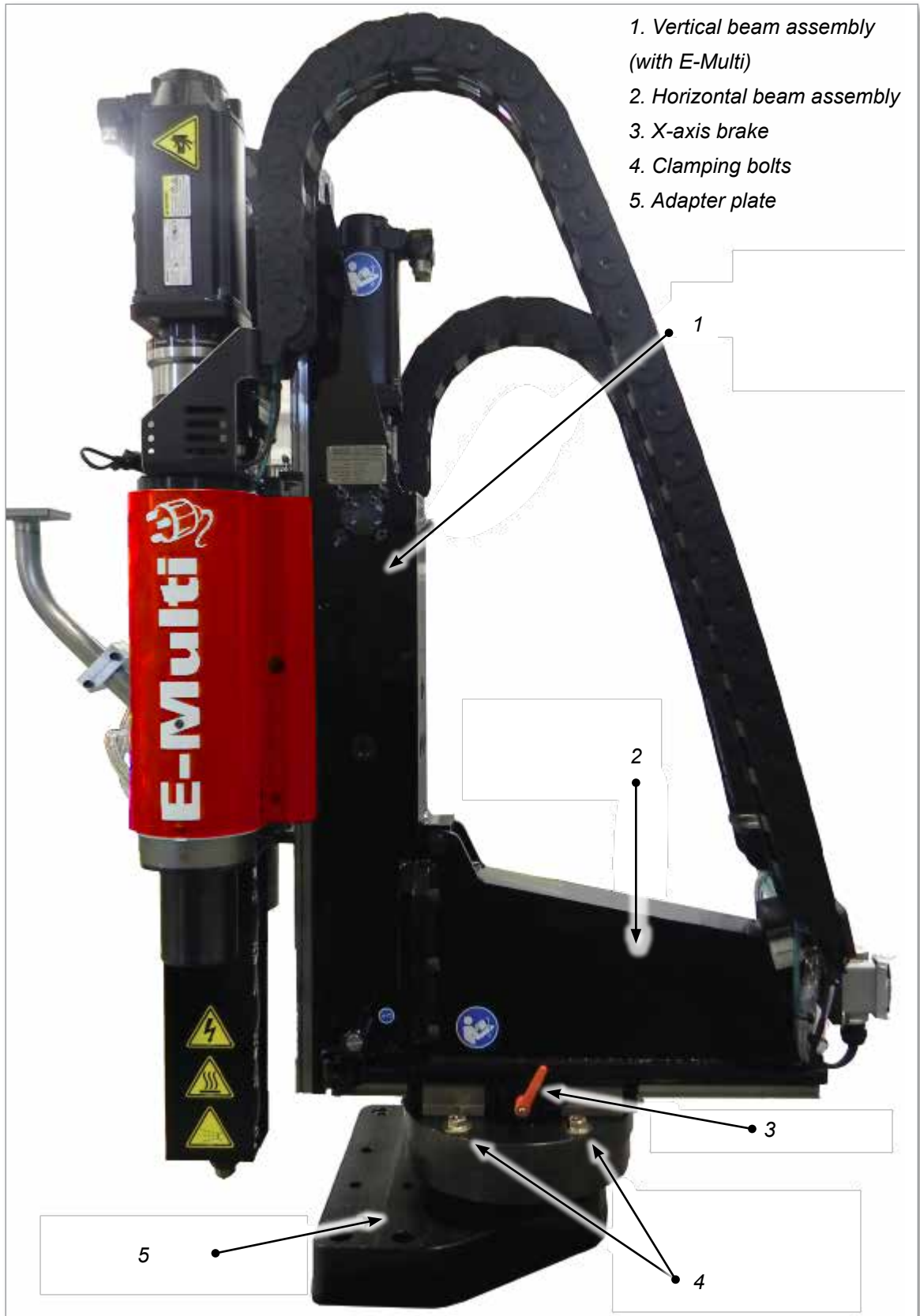
Figure 11-1 Main components of the E-Multi Radial
