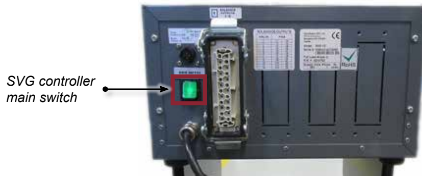
Figure 6-2 SVG controller main switch
