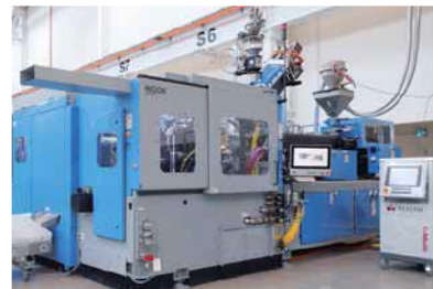
Niigon 150NPET with a 32 cavity co-injection hot runner and E-Multi from Mold-Masters.
