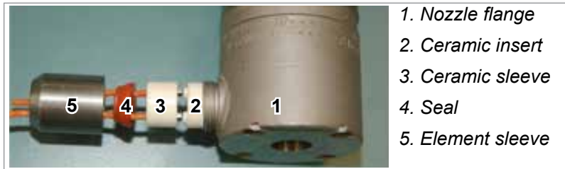
Figure 11-6 Nozzle terminal assembly
