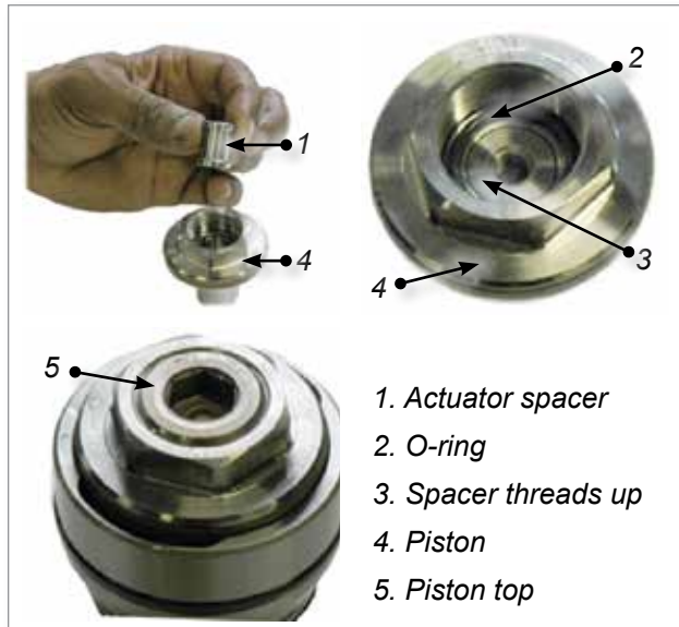
Figure 10-15 Piston spacer installation
