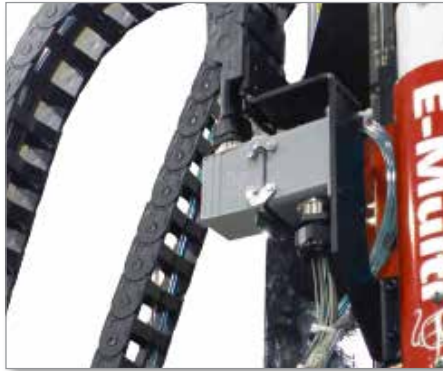
Figure 11-7 Install the barrel heats connector
