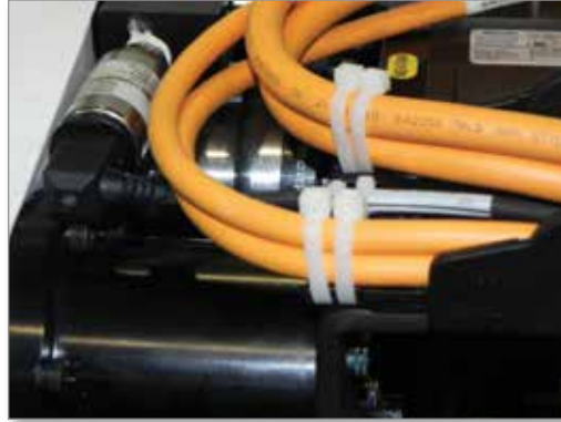
Figure 7-2 Cables held with wire ties
