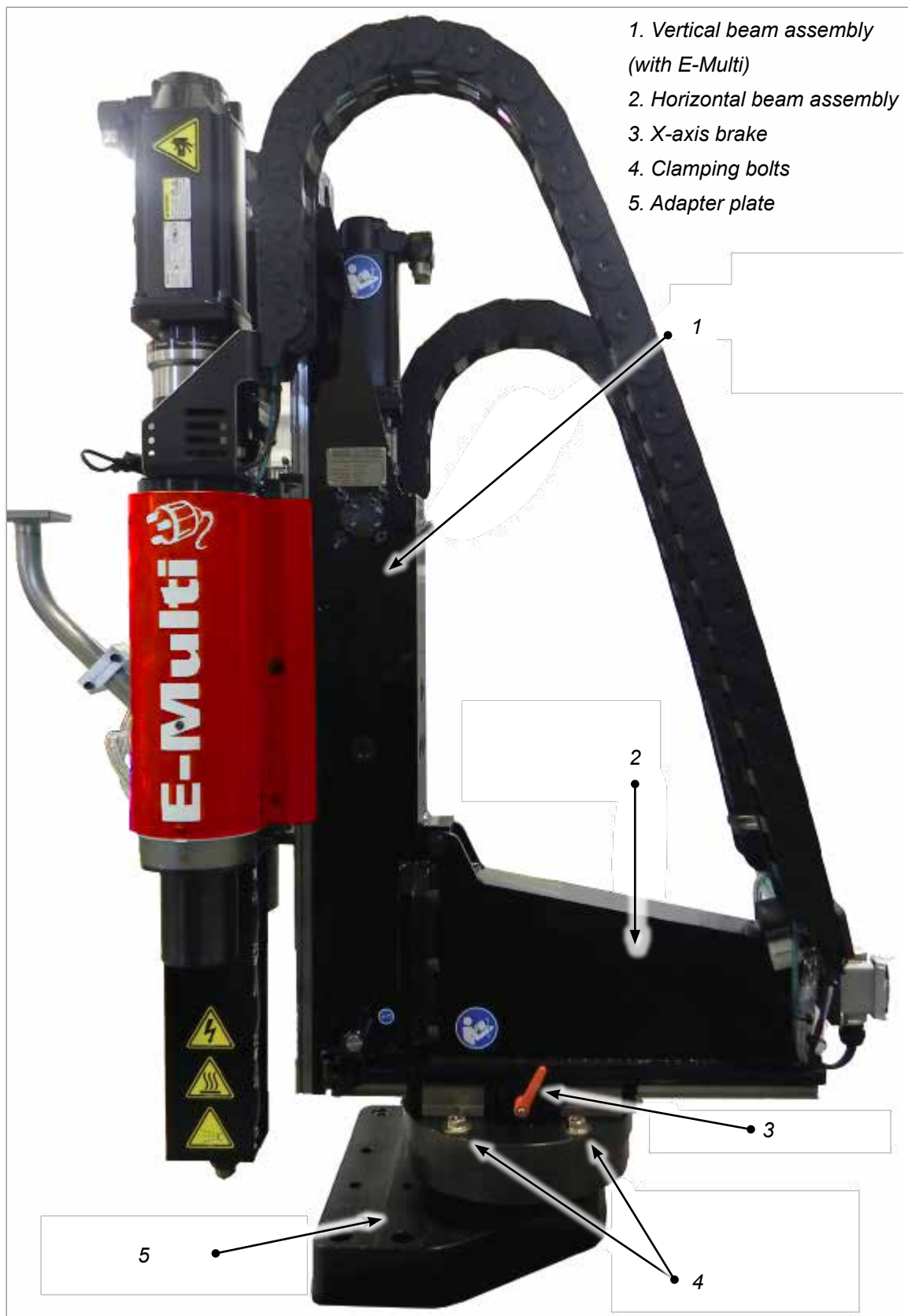
Figure 11-1 Main components of the E-Multi Radial
