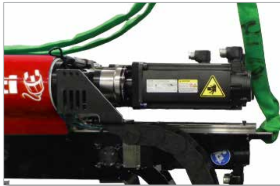
Figure 11-4 Rear sling attachment
