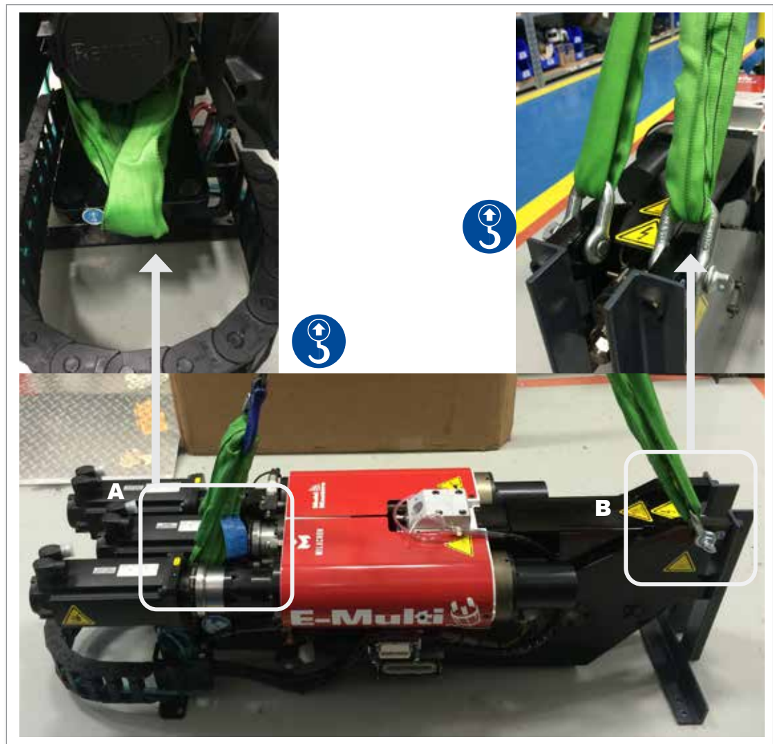
Figure 3-7 EM3 horizontal lift connections. EM1 / EM2 similar
