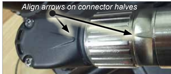
Figure 7-3 Correct connector alignment
