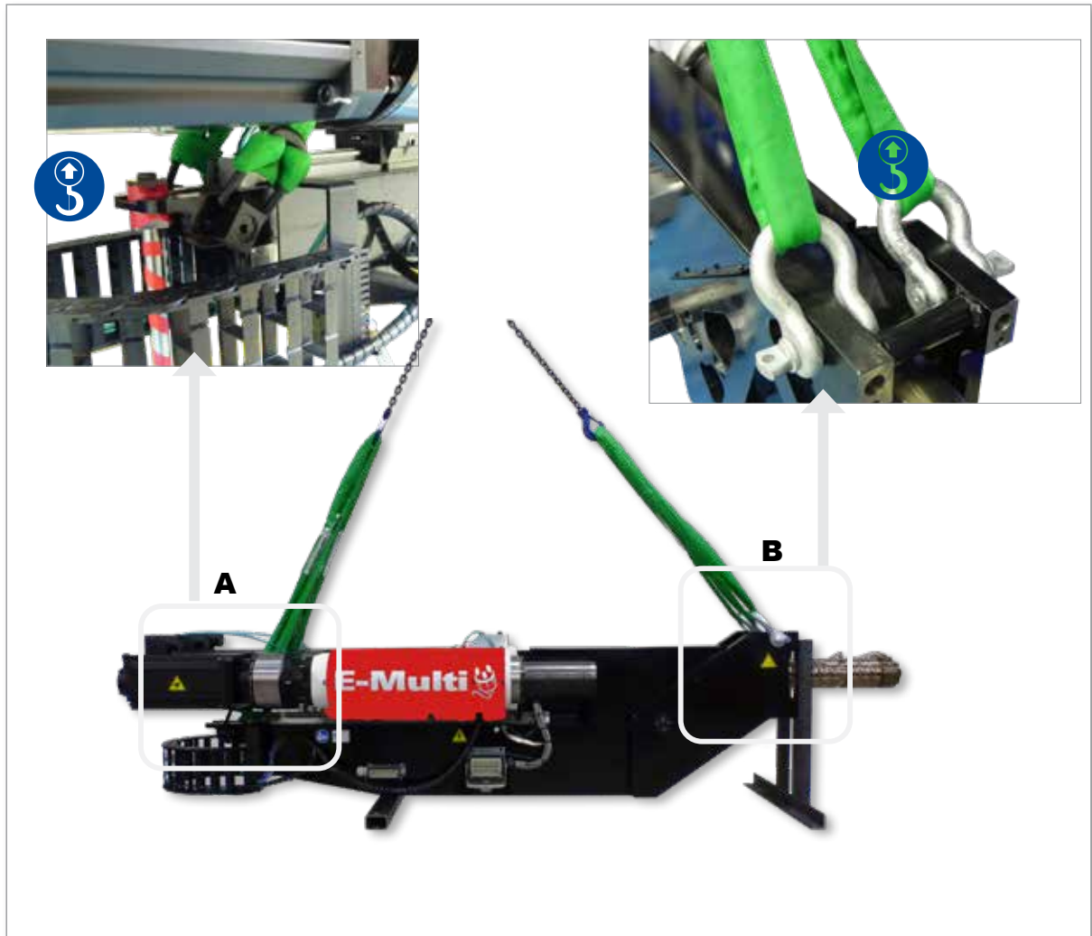
Figure 3-8 EM4 horizontal lift connections
