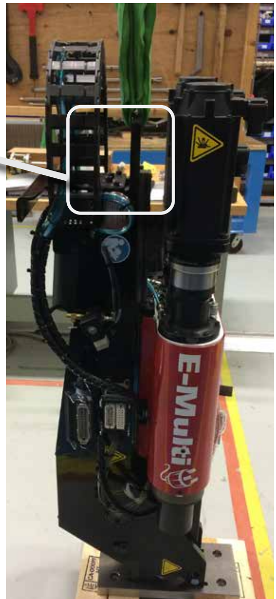
Figure 3-6 EM1 / EM2 vertical lifting connections (EM3 similar)
