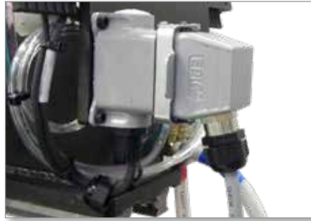
Figure 11-9 Install the I/O connector
