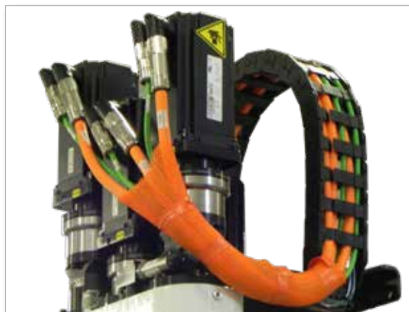
Figure 7-1 EM3 Servo cable routing
