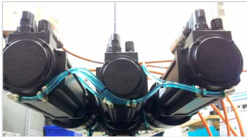
Figure 7-7 EM3 / EM4 Servo motor cooling connections
