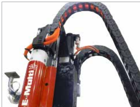
Figure 11-8 Attach the servo motor cables
