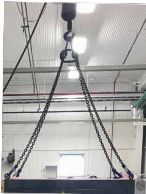
Figure 3-11 Attach slings to all four eyebolts
