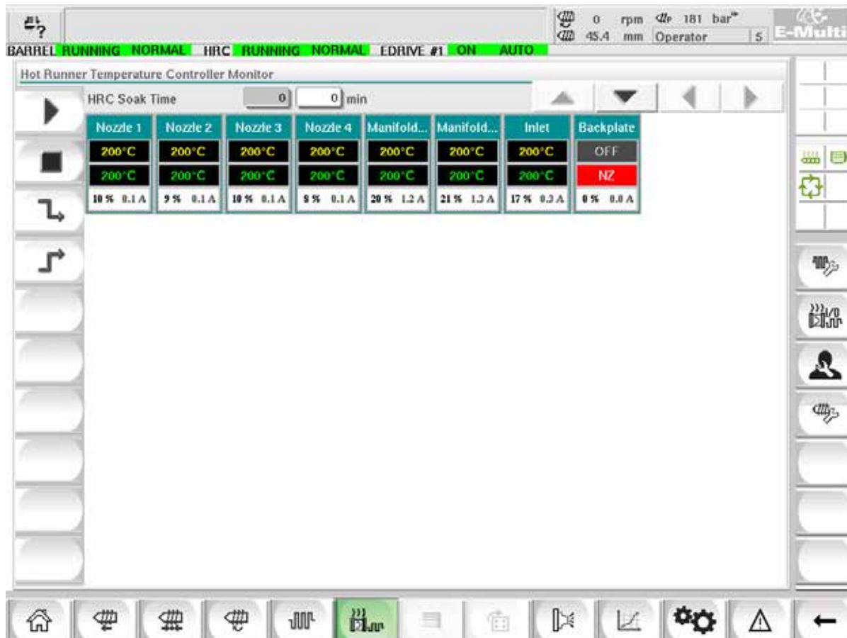
Figure 7-10 Hot runner controller monitor screen
