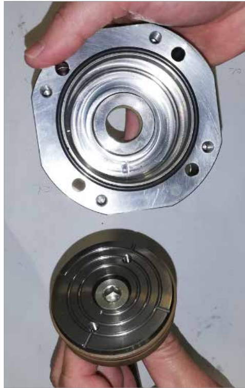
Figure 4-15 Install the piston
