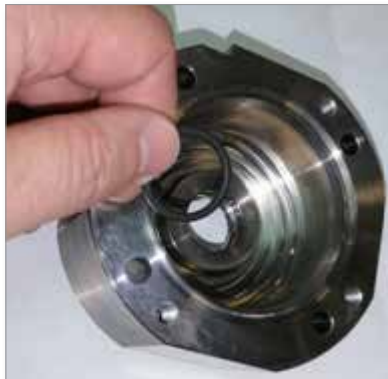
Figure 4-9 Install O-ring for rod seal
