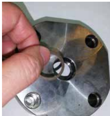
Figure 4-13 Install wiper seal
