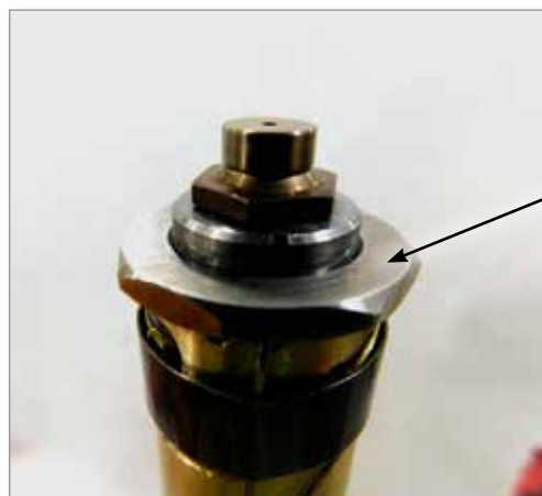
Figure 5-8 Nozzle center guiding ring
