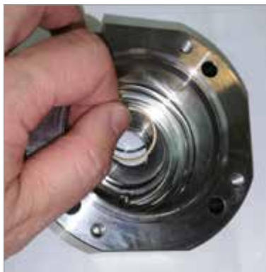
Figure 4-10 Install rod seal
