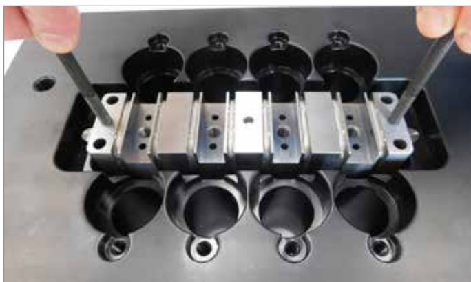
Figure 19-20 Install Melt-CUBE manifold
