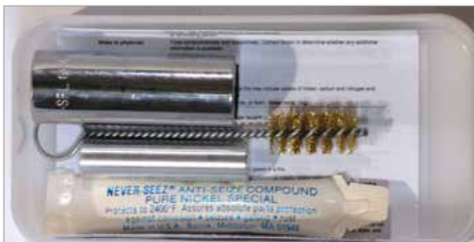
Figure 15-10 Sprint gate seal tools
