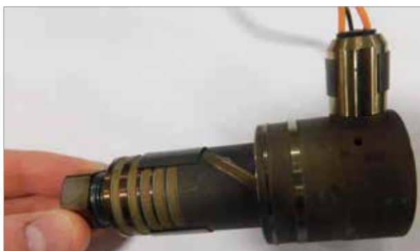
Figure 19-16 Install the top half of the melt transfer link
