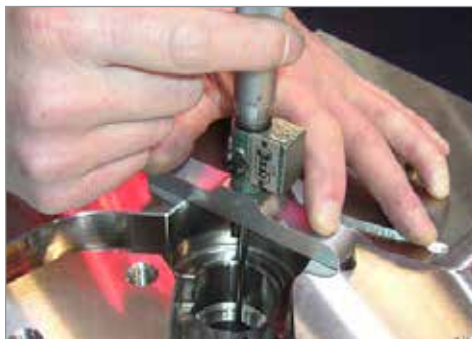
Figure 5-27 Calculating nozzle bore depth "a"
