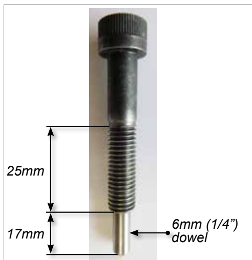
Figure 19-7 M10-1.5 jack bolt (SHCSM10X50-A)
