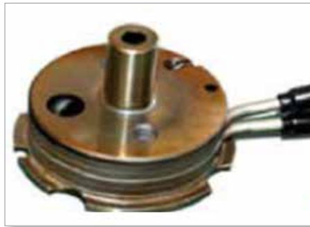
Figure 5-16 Heated valve bushing
