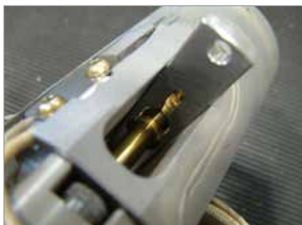
Figure 17-2 Accu-Line™ valve pin holder and valve pin
