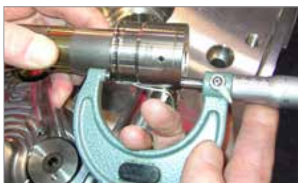
Figure 5-28 Calculating nozzle flange height "b"
