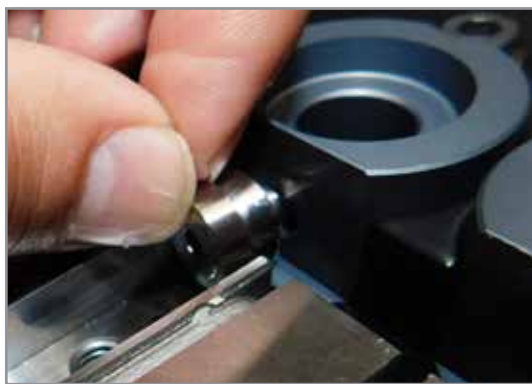
Figure 19-25 Install gate seal
