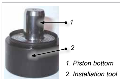
Figure 10-6 Piston bottom with installation tool
