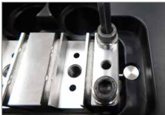
Figure 19-21 Install washers and bolts
