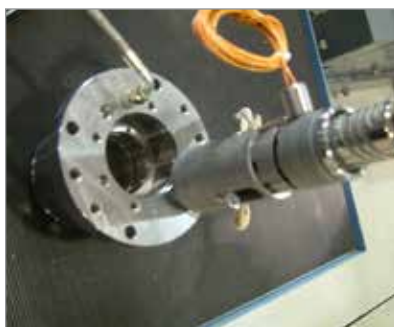
Figure 17-2 Accu-Line™ valve pin holder and valve pin
