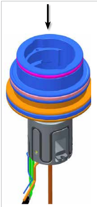
Figure 11-12 Install piston assembly onto heated body
