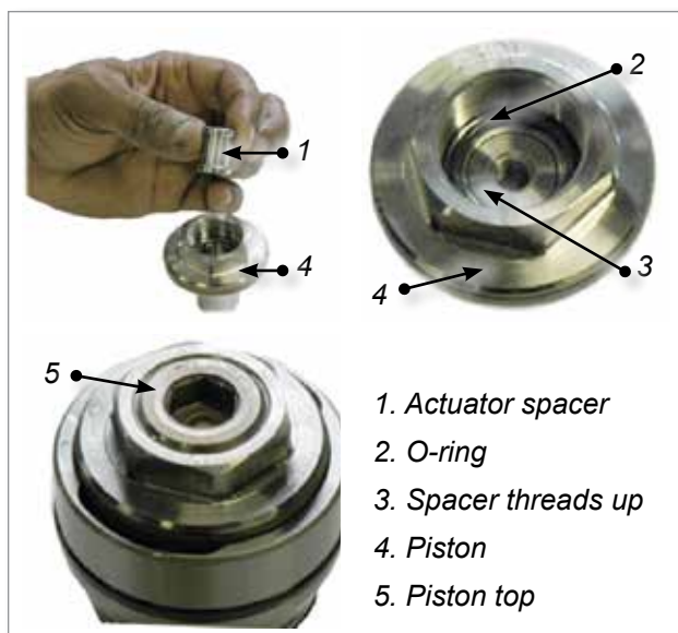
Figure 10-19 Piston spacer installation
