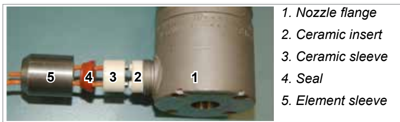
Figure 15-6 Nozzle terminal assembly
