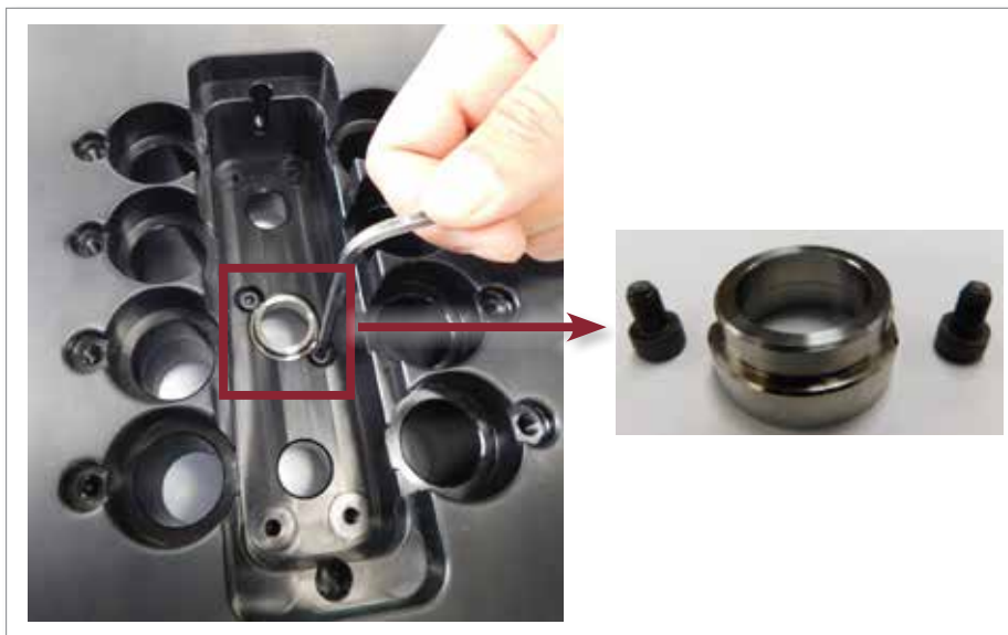
Figure 19-18 Install the center locator
