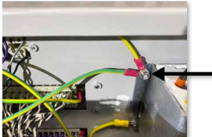
Figure 3-2 Ground connection of the Me controller
