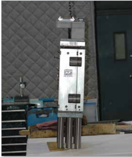
Figure 3-6 Align wooden block beneath the plate or mold
