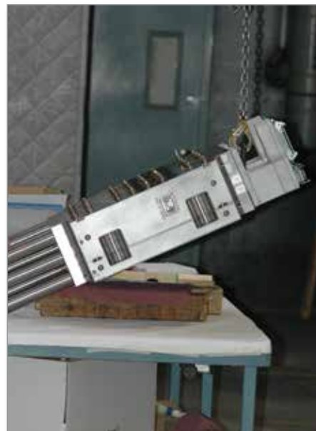
Figure 3-8 Wooden blocks beneath plate or mold as required
