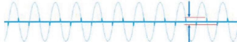
Phase Angle Firing (requires a fast, dedicated CPU) Controller begins soft start at very low voltage levels, eliminating the possibility of heater arc over.
