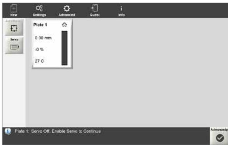
Figure 4-2 Main screen of the E-Drive controller
