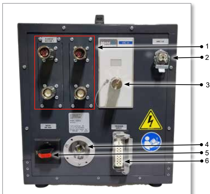
Figure 4-1 Connections of the E-Drive cabinet
