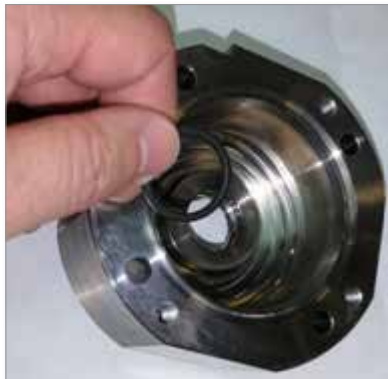
Figure 4-9 Install O-ring for rod seal
