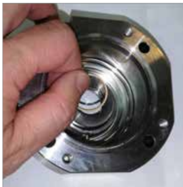
Figure 4-10 Install rod seal
