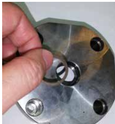
Figure 4-13 Install wiper seal
