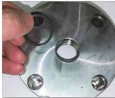
Figure 4-12 Install O-ring for wiper seal
