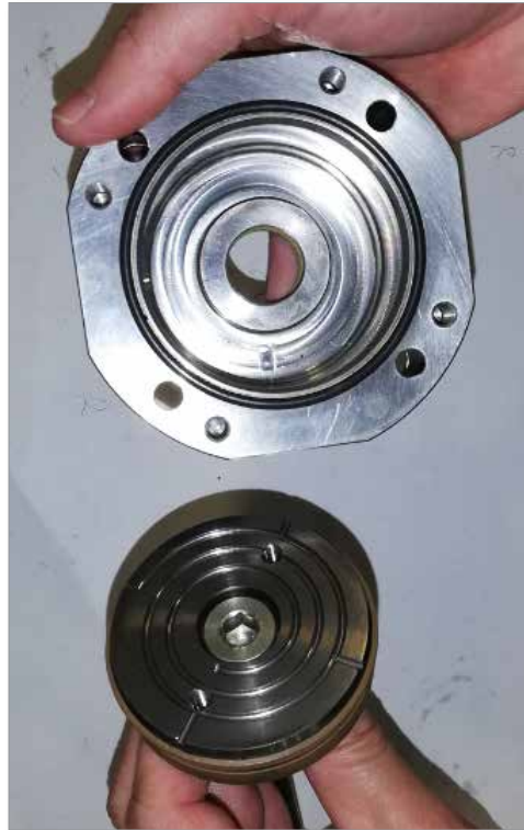
Figure 4-15 Install the piston
