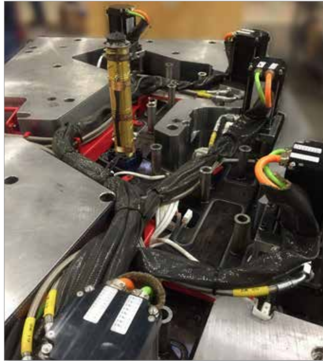
Figure 6-12 Attach cables to wiring channel
