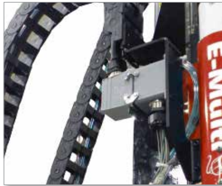
Figure 11-7 Install the barrel heats connector
