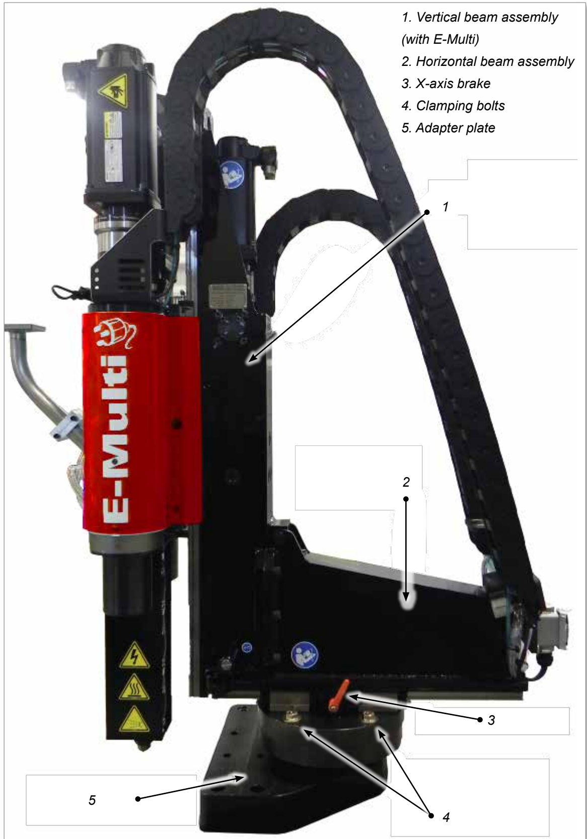
Figure 11-1 Main components of the E-Multi Radial
