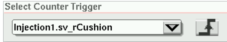
Figure 8-3 Rising edge trigger
