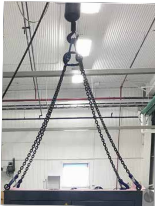
Figure 3-11 Attach slings to all four eyebolts
