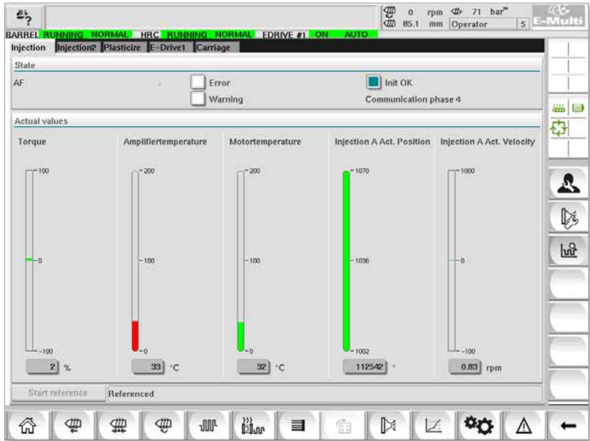
Figure 7-34 Drive monitor screen
