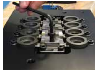
STEP 1 Remove bolt & rectangular washer
