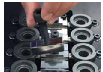
STEP 2 Extract melt block using an M10 bolt
