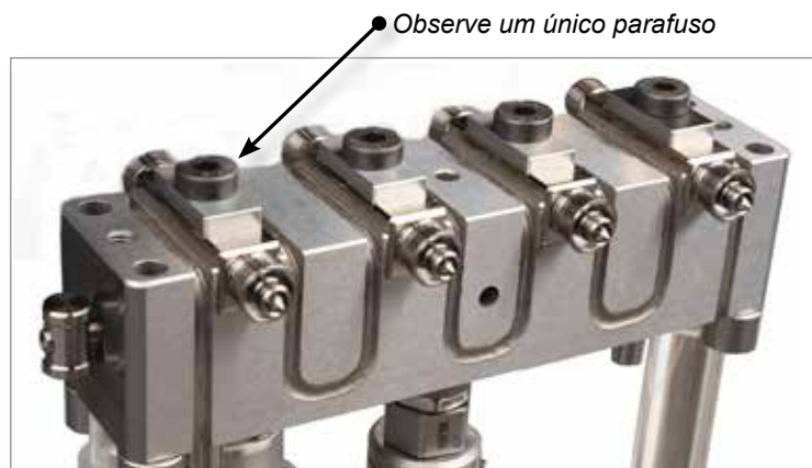
Figura 5-79 Design B do Melt-Cube
