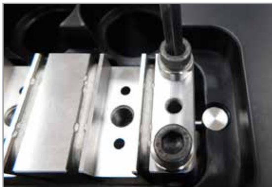
Figura 5-98 Instale as arruelas e os parafusos
