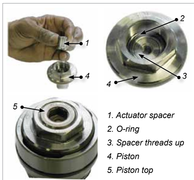
Figure 5-53 Piston spacer installation
