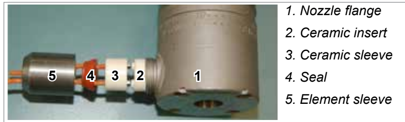
Figure 10-6 Nozzle terminal assembly
