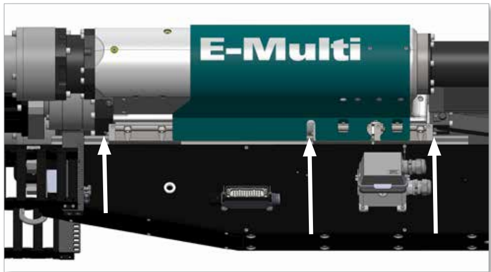
Figure 9-23 Side view showing locations of linear-guide lubrication points (3)
