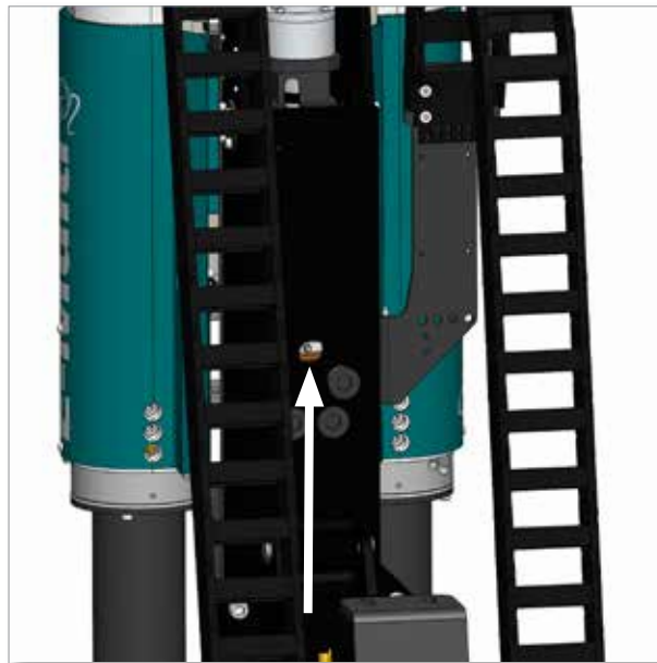
Figure 9-4 Carriage ball screw lubrication point (1)
