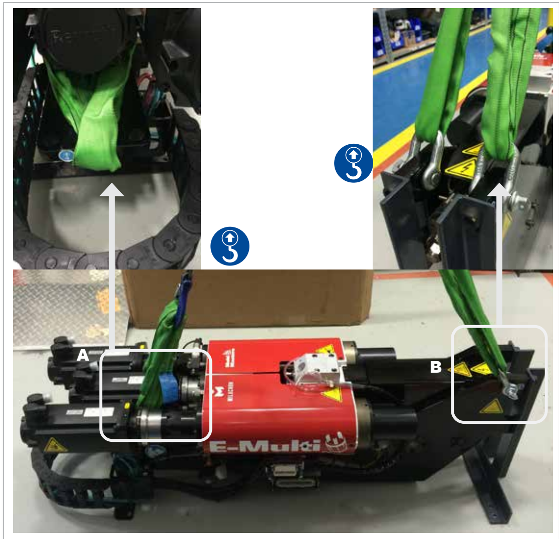
Figure 3-7 EM3 horizontal lift connections. EM1 / EM2 similar
