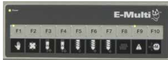
Figure 8-2 Button strip below controller display (HMI)
