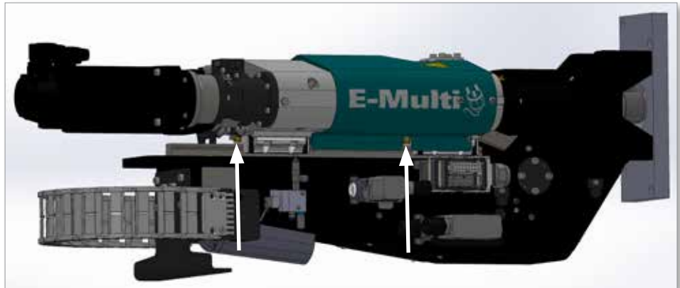
Figure 9-2 Linear guide lubrication points (2)
