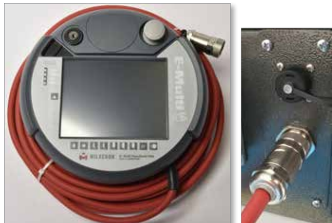
Figure 7-5 Hand-held HMI and connection
