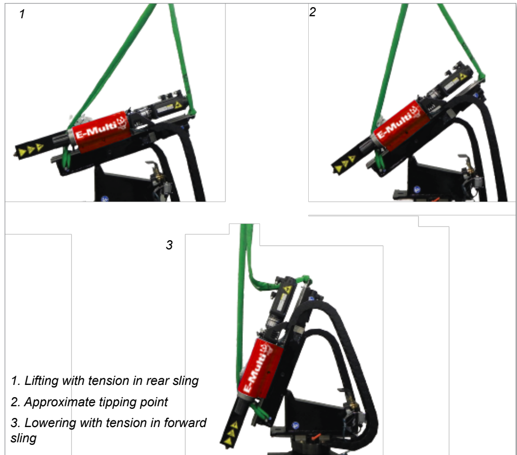
Figure 12-6 Tilting the E-Multi Radial from the horizontal to vertical position
