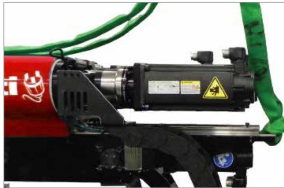
Figure 12-4 Rear sling attachment
