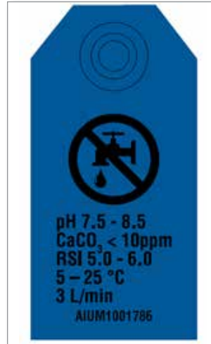
Figure 7-1 Water quality specification tag on E-Multi
