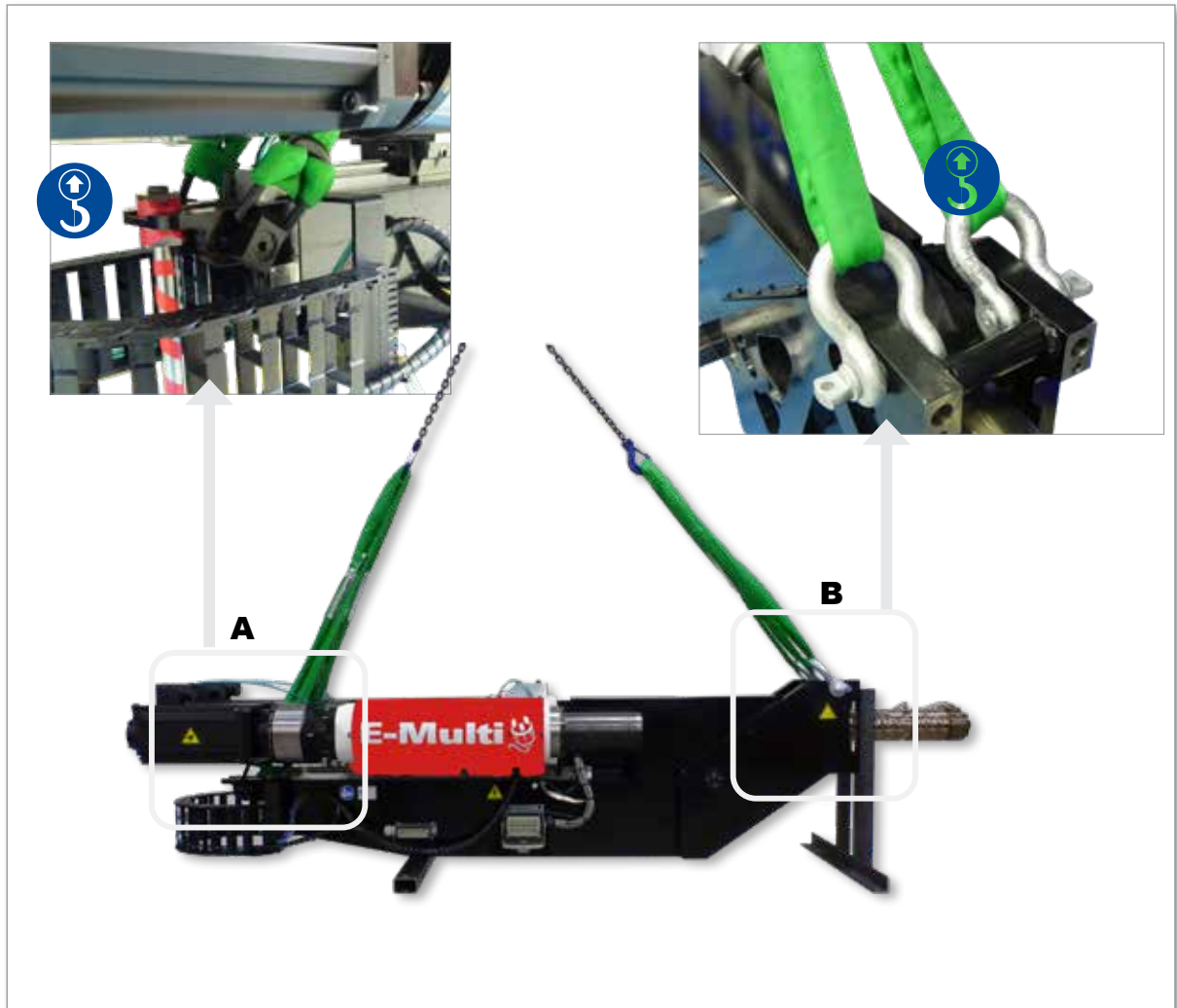
Figure 3-8 EM4 horizontal lift connections
