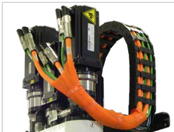
Figure 7-1 EM3 Servo cable routing
