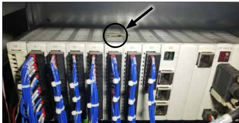
Figure 9-5 Location of the CMOS battery tray (newer cabinets)
