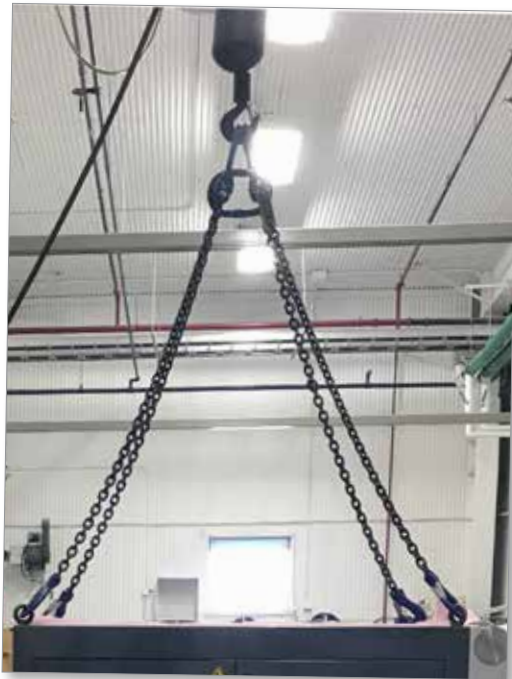
Figure 3-11 Attach slings to all four eyebolts
