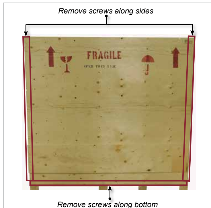
Figure 3-8 Remove screws from side and bottom
