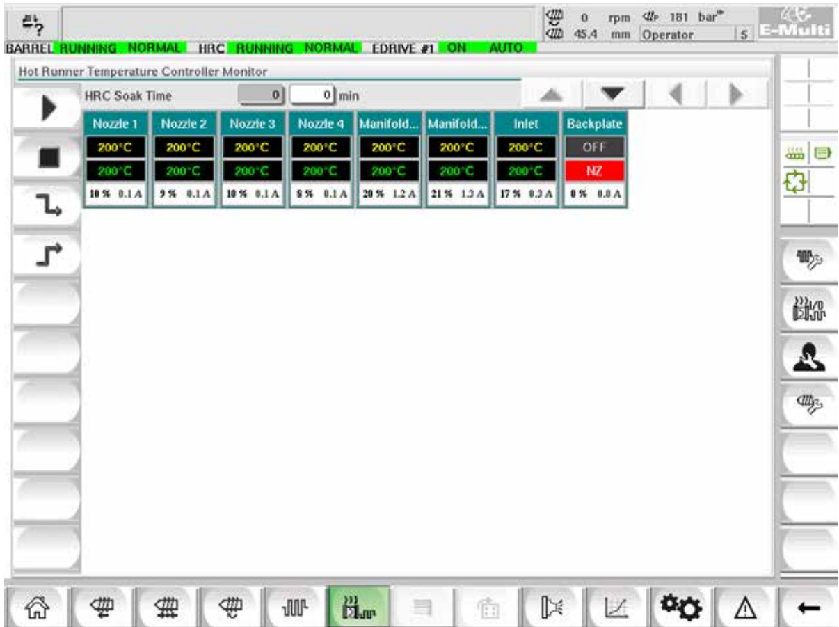
Figure 7-11 Hot runner controller monitor screen
