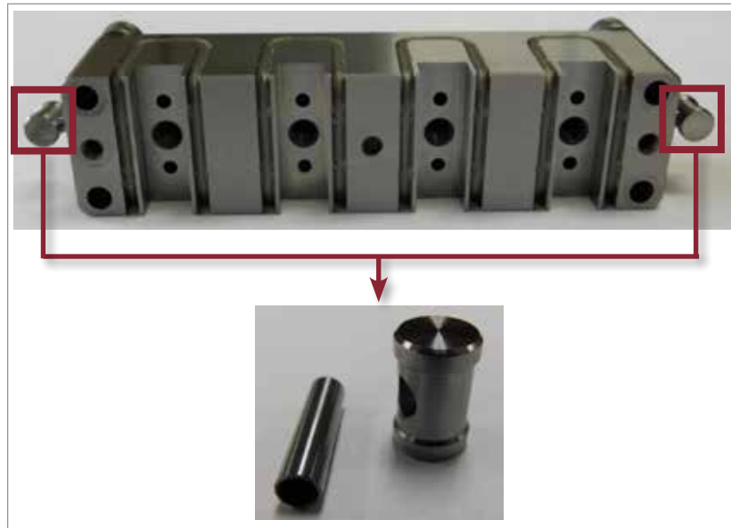
Figure 5-94 Install the anti-rotation dowel
