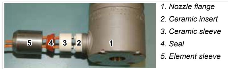
Figure 10-6 Nozzle terminal assembly
