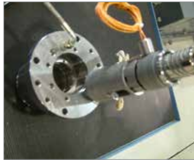
Figure 5-69 Accu-Line valve pin holder and valve pin
