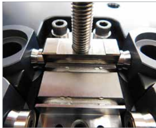
Figure 5-106 Extract the melt block
