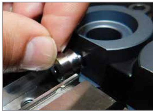
Figure 5-102 Install gate seal
