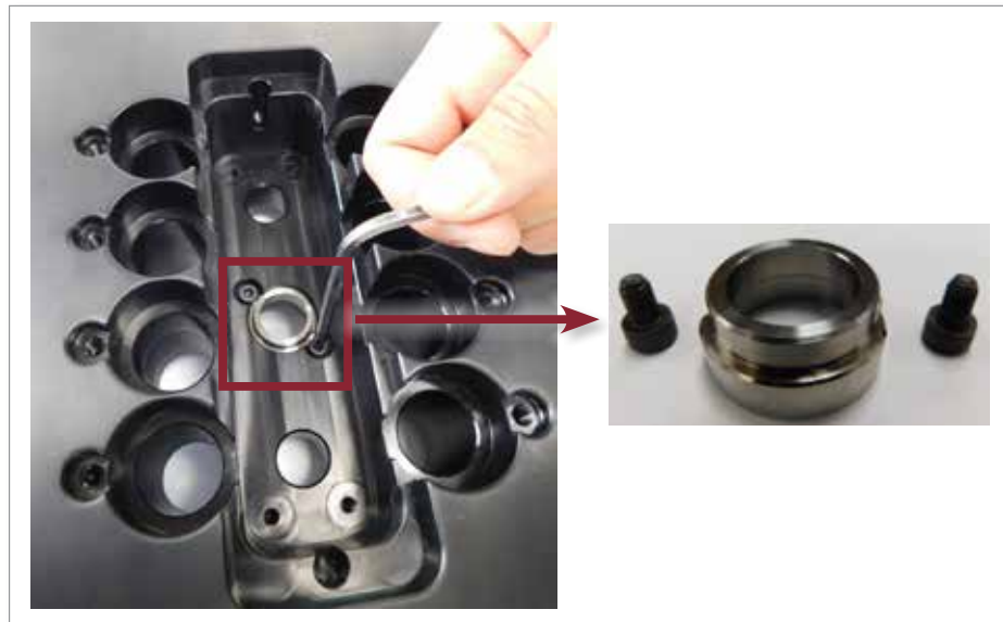
Figure 5-95 Install the center locator
