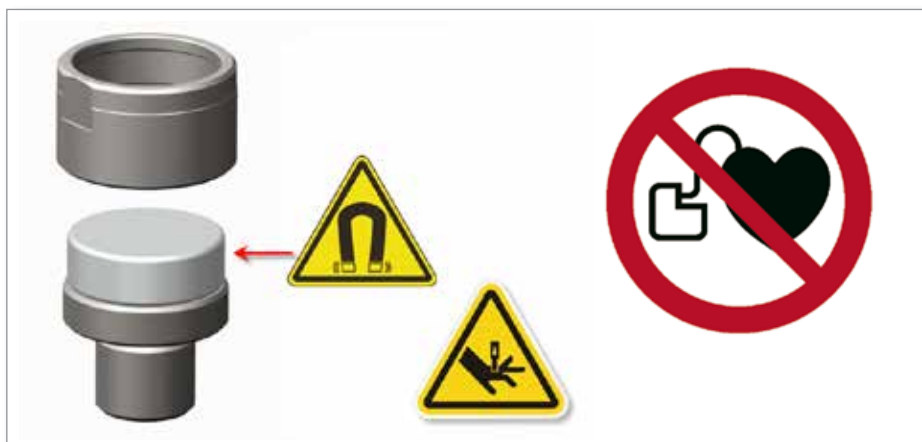
Figure 5-65 Mag-Pin safety hazards
