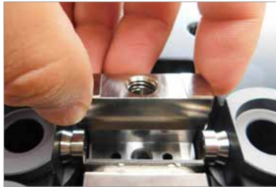
Figure 5-104 Install by hand
