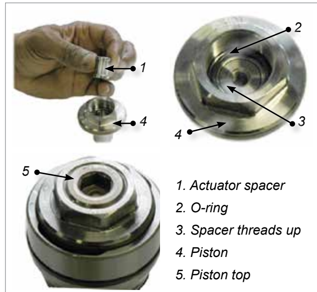
Figure 5-53 Piston spacer installation
