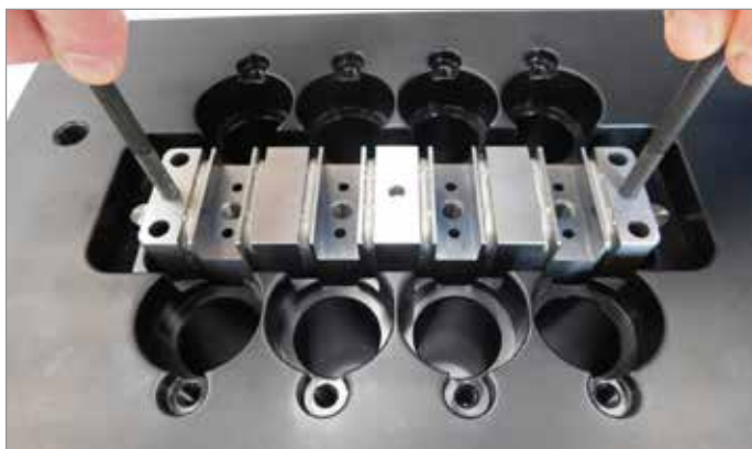
Figure 5-97 Install Melt-Cube manifold
