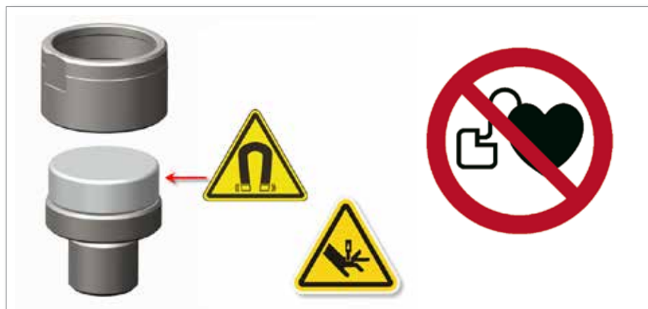
Figure 5-65 Mag-Pin safety hazards
