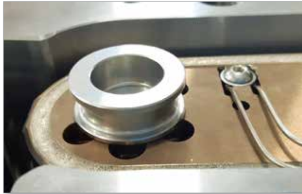
Figure 5-24 Support bushing for systems with MasterShield
