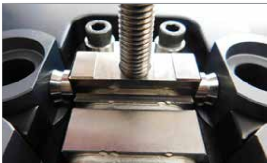
Figure 5-103 Install with an M10 lifting bolt
