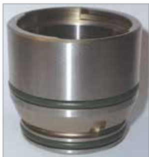
Figure 5-38 6X00 Series and 7100 Series bottom cylinder O-rings
