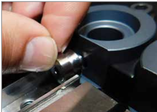
Figure 5-102 Install gate seal
