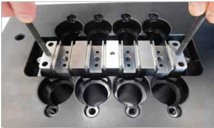
Figure 5-97 Install Melt-Cube manifold
