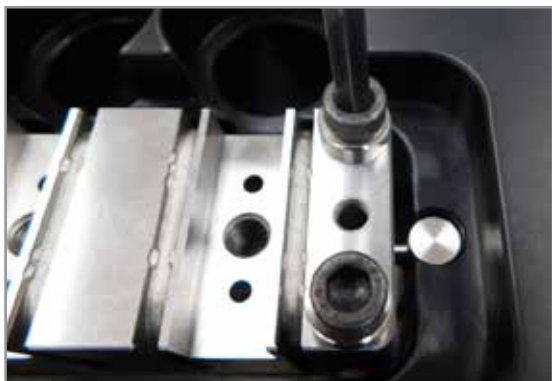
Figure 5-98 Install washers and bolts
