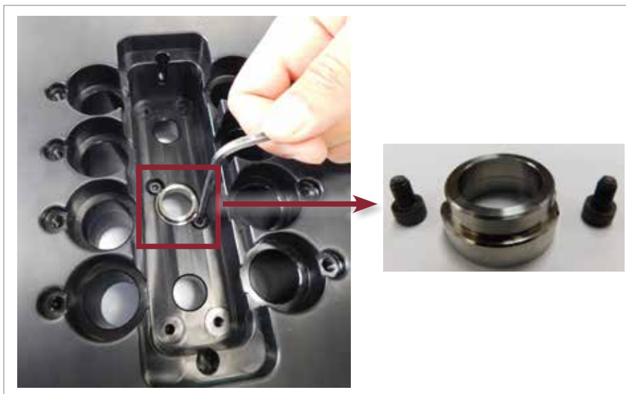
Figure 5-95 Install the center locator
