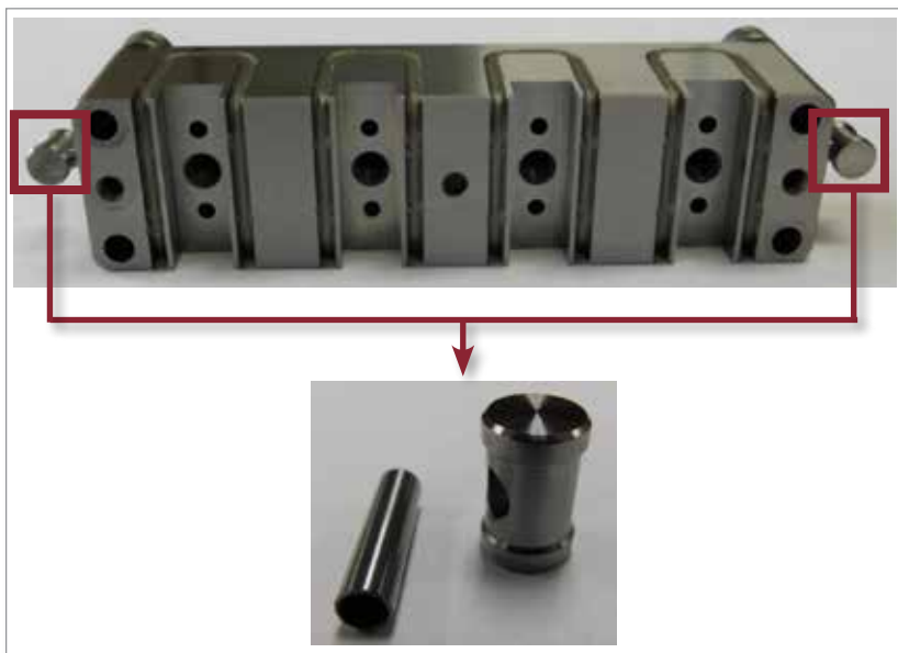
Figure 5-94 Install the anti-rotation dowel
