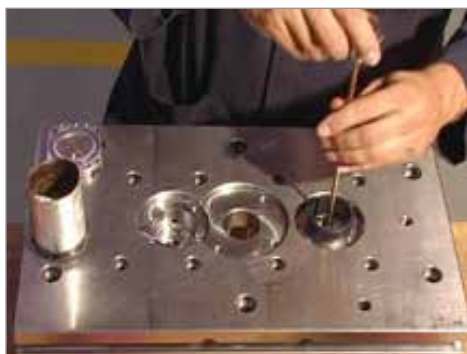
Figure 5-54 Valve pin and piston installation
