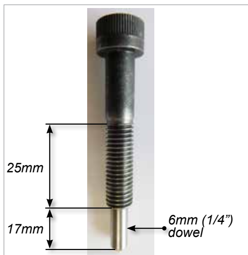
Figure 5-84 M10-1.5 jack bolt (SHCSM10X50-A)
