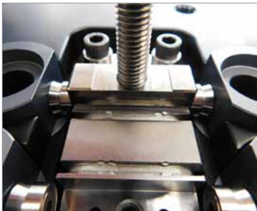
Figure 5-106 Extract the melt block
