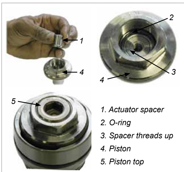
Figure 5-53 Piston spacer installation
