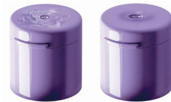
Fig. 4. Cloudy appearance on a highly polished surface, as with this violet hinged lid closure, is a phenomenon caused by flow lines. After the changeover to Apex, the cloudy appearance was eliminated without process modification. © Mold-Masters
