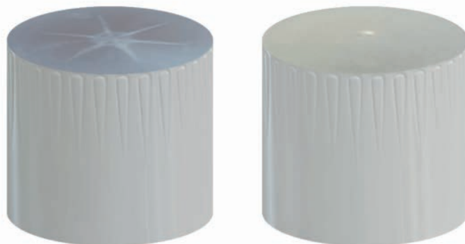
Fig. 5. Flow lines on the satin-finish screw cap of a "premium personal care" product (left). The use of the Apex gate has completely eliminated the flow lines (right). © Mold-Masters
