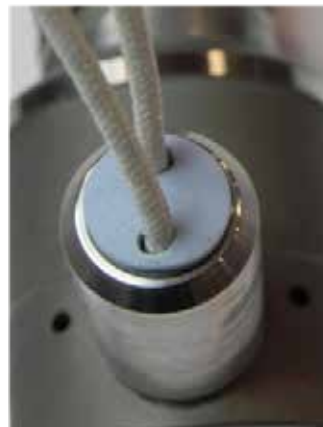
Figure 11-2 Nozzle terminal assembly
