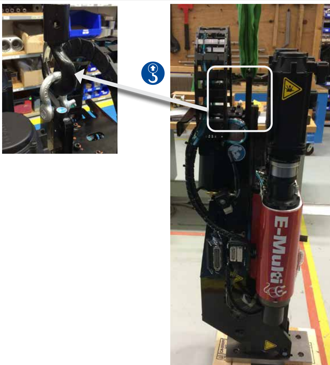
Figure 3-6 EM1 / EM2 vertical lifting connections (EM3 similar)
