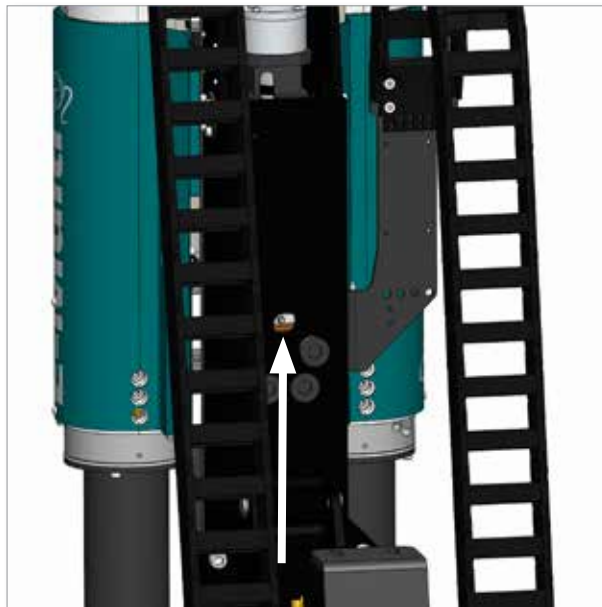
Figure 9-4 Carriage ball screw lubrication point (1)
