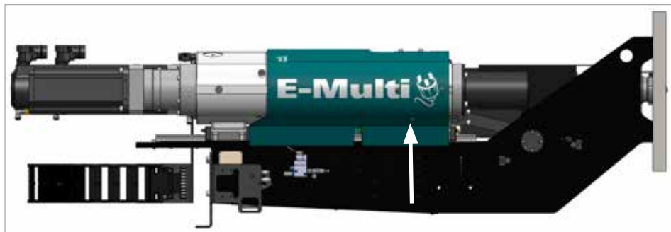
Figure 9-14 Side view showing location of ball-screw lubrication points
