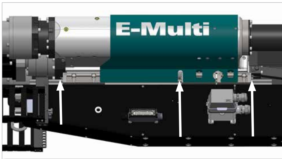
Figure 9-23 Side view showing locations of linear-guide lubrication points (3)
