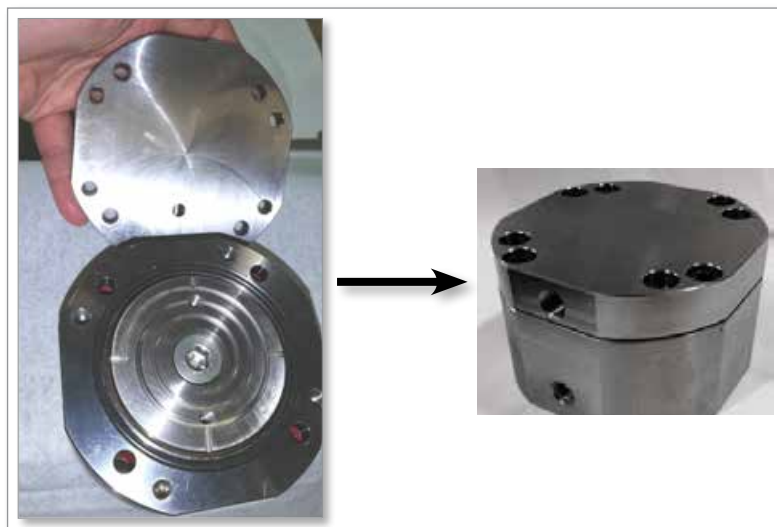
Figure 4-21 Assembled cylinder - note ports
