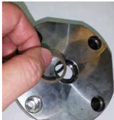
Figure 4-17 Install wiper seal
