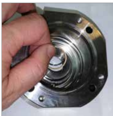
Figure 4-14 Install rod seal
