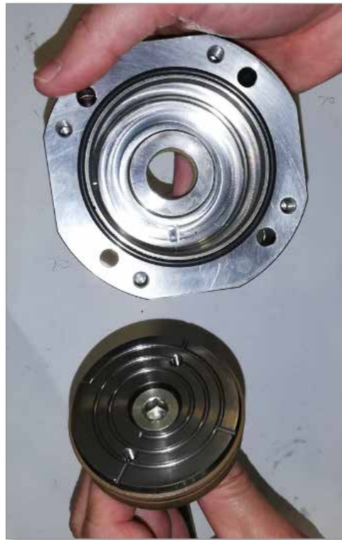
Figure 4-19 Install the piston
