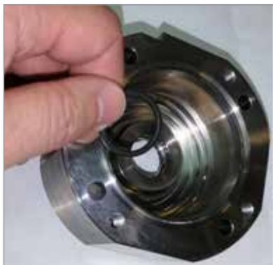
Figure 4-13 Install O-ring for rod seal
