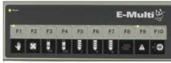
Figure 6-2 Button strip below controller display (HMI)
