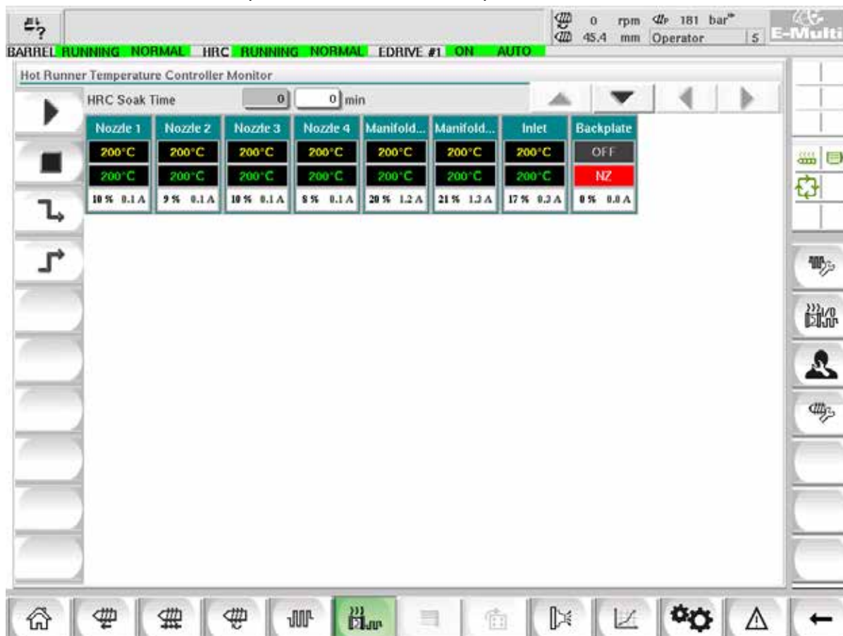
Figure 7-11 Hot runner controller monitor screen
