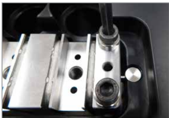
Figure 5-97 Install washers and bolts
