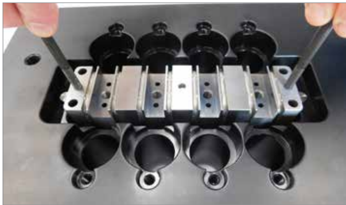
Figure 5-96 Install Melt-Cube manifold
