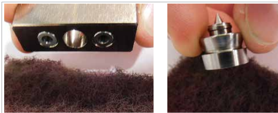
Figure 5-107 Clean the melt block and gate seal
