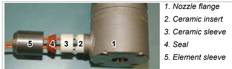
Figure 10-6 Nozzle terminal assembly
