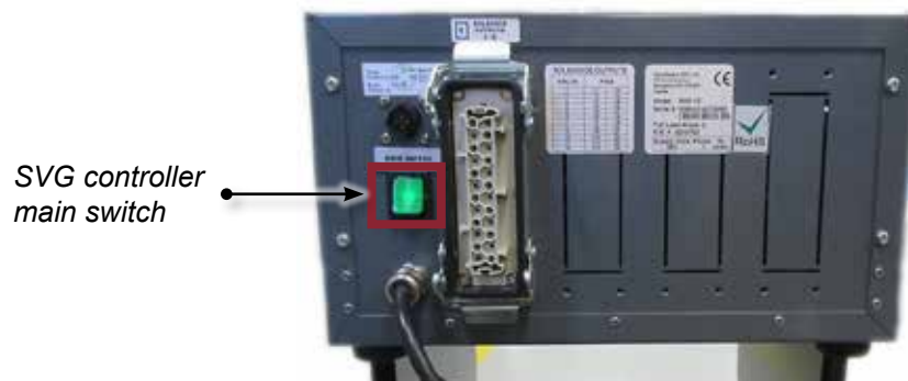
Figure 6-2 SVG controller main switch
