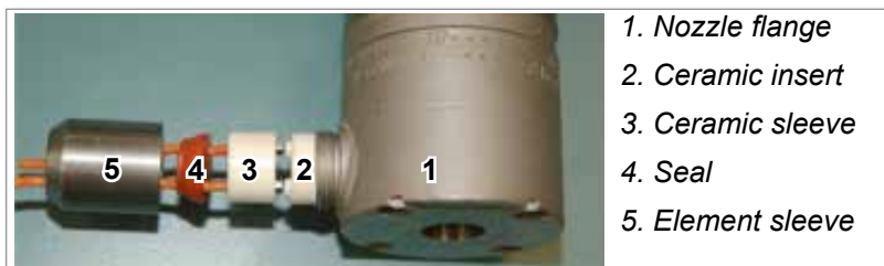
Figure 10-6 Nozzle terminal assembly
