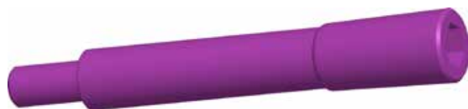
Figure 5-112 Speed-LOK center bolt (torque: 7.34–9.60 Nm (65–85 in-lb))
