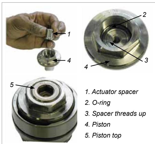
Figure 5-52 Piston spacer installation
