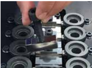
STEP 2 Extract melt block using an M10 bolt
