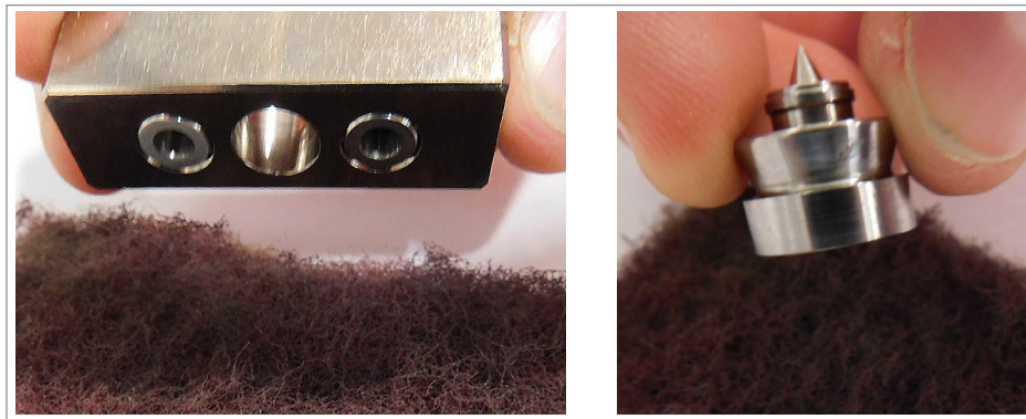
Figure 5-107 Clean the melt block and gate seal
