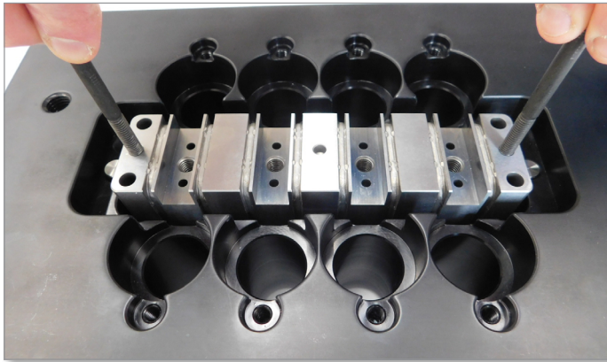
Figure 5-96 Install Melt-Cube manifold
