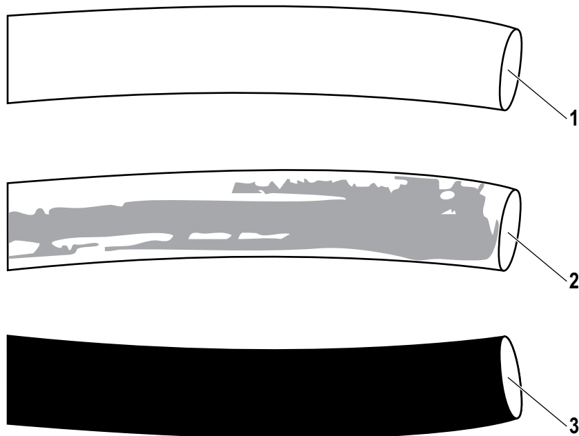
Figure 11-1 Comparison of clean and contaminated cooling lines
