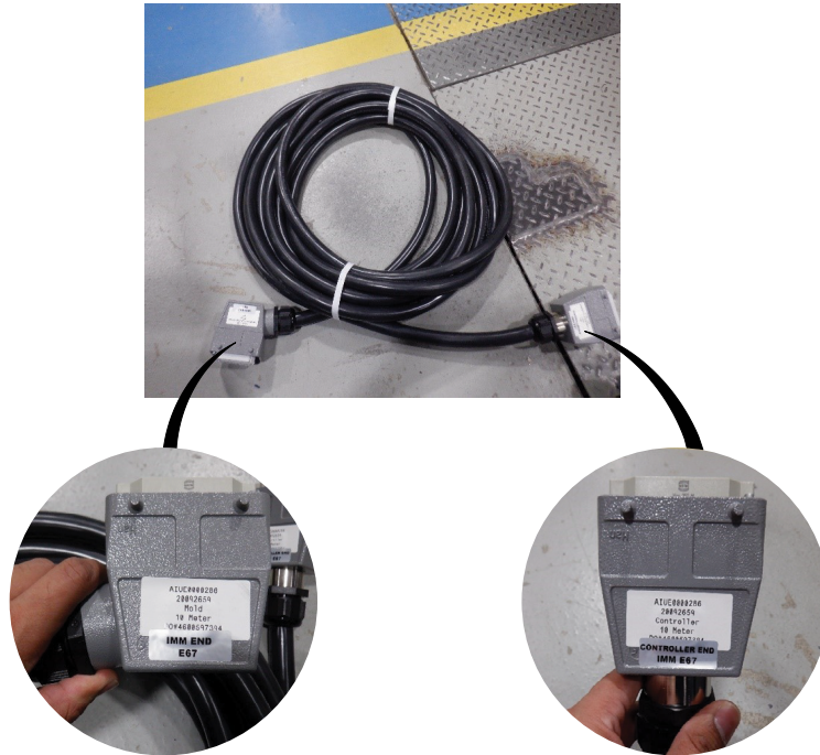
Figure 5-5 IMM E67 cable with mold/IMM end and controller end
