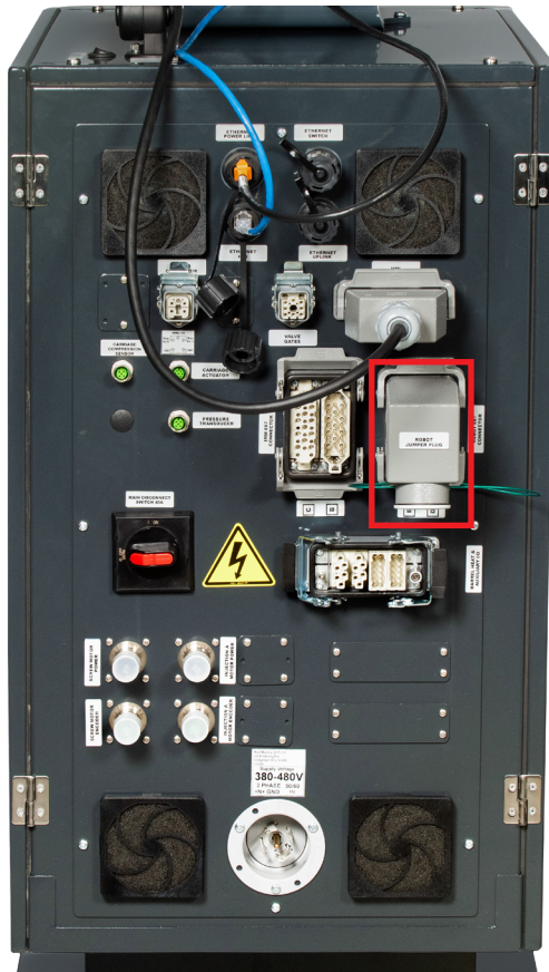
Figure 5-2 Robot jumper plug
