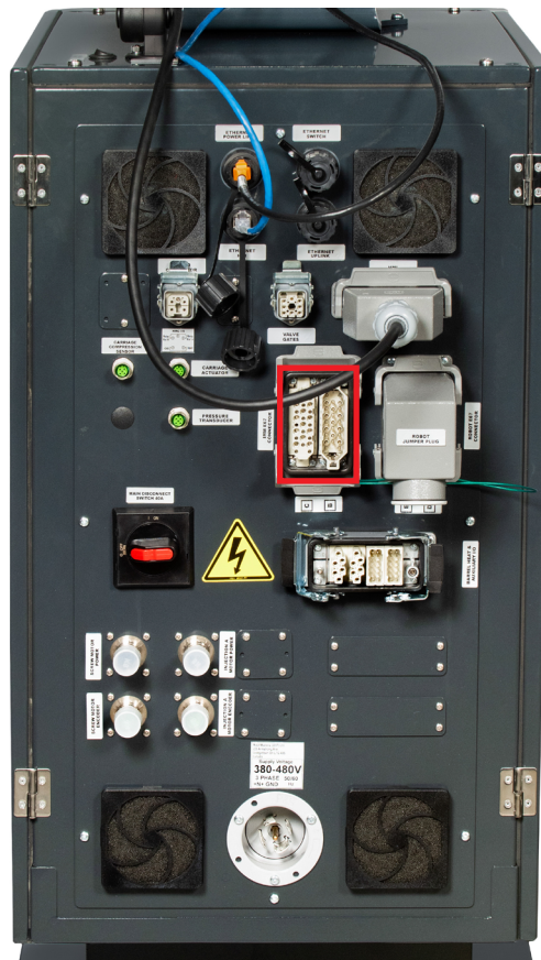
Figure 5-6 IMM E67 connector on the back of the controller
