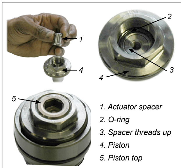
Figure 5-52 Piston spacer installation
