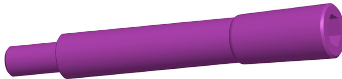
Figure 5-112 Speed-LOK center bolt (torque: 7.34–9.60 Nm (65–85 in-lb))
