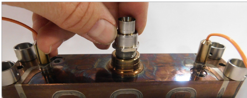
Figure 5-91 Install the bottom half of the melt transfer link
