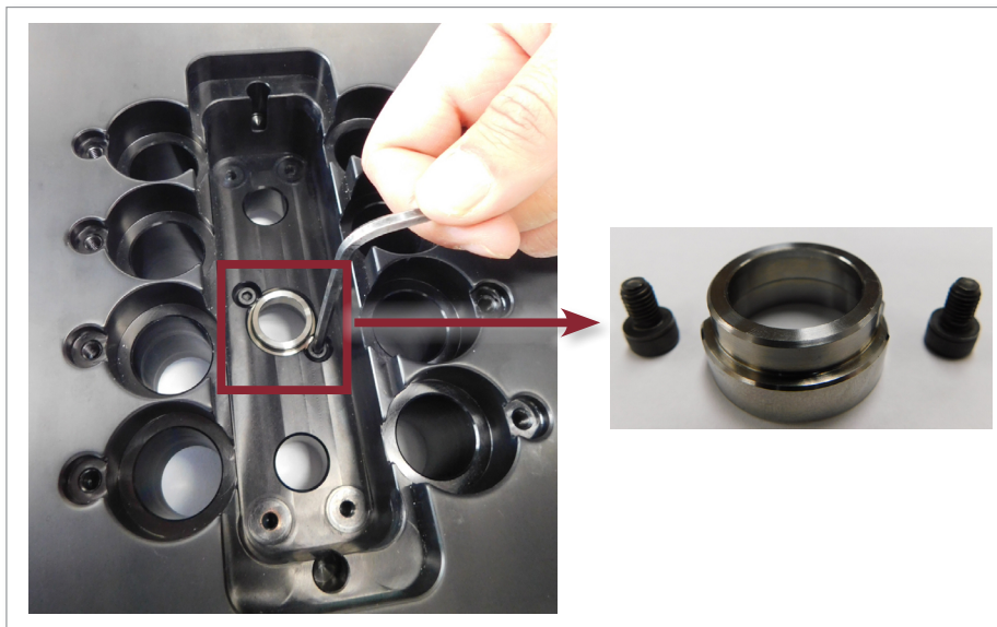
Figure 5-94 Install the center locator
