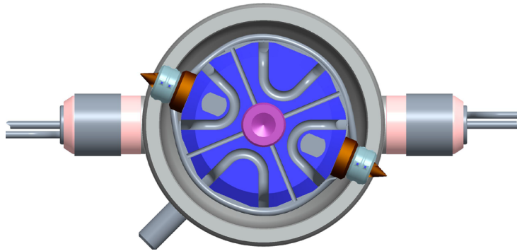
Figure 5-108 Two-tip DeXa nozzle (bottom view)
