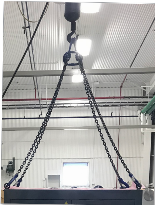
Figure 3-11 Attach slings to all four eyebolts
