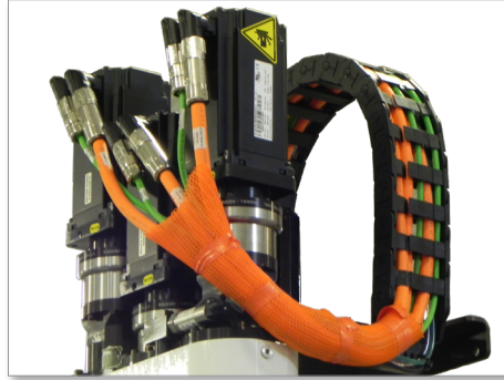
Figure 5-1 EM3 servo cable routing
