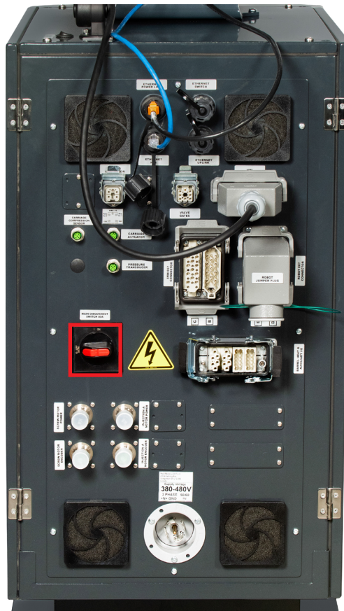
Figure 6-1 Main power switch
