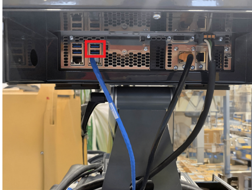
Figure 10-13 USB connections on the bottom of the touchscreen
