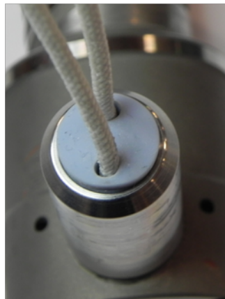
Figure 11-2 Nozzle terminal assembly
