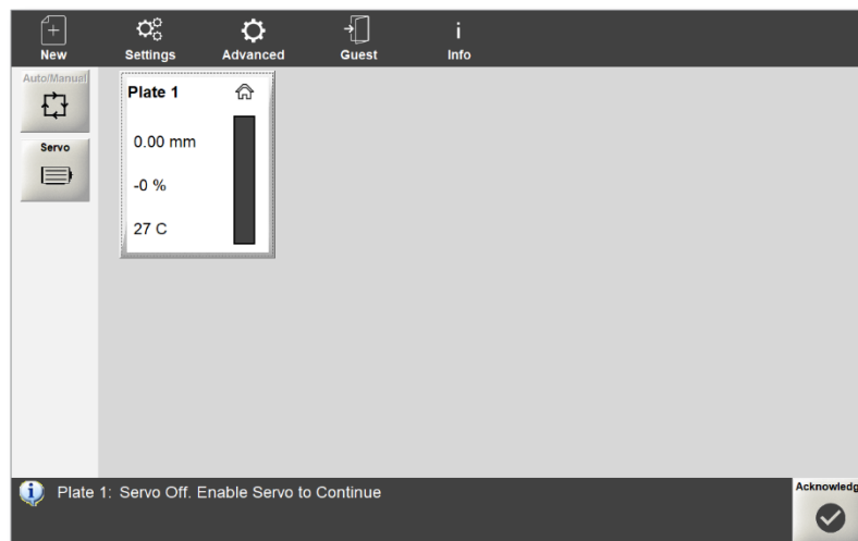
Figure 7-2 Main screen of the E-Drive controller
