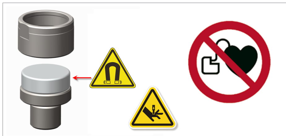
Figure 5-1 Mag-Pin safety hazards
