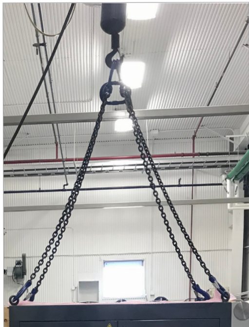
Figure 3-11 Attach slings to all four eyebolts
