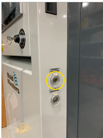
Figure 5-6 Ethernet port on controller
