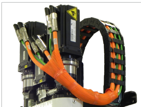
Figure 5-1 EM3 servo cable routing
