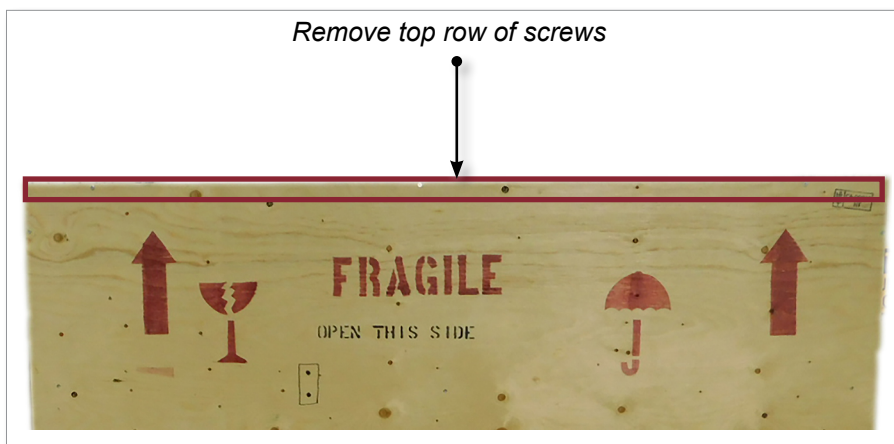
Figure 3-6 Remove top row of screws
