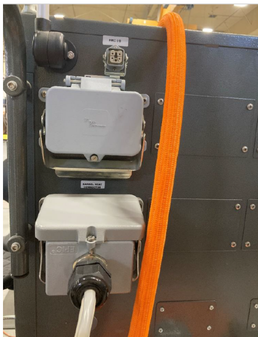
Figure 8-41 Controller back with barrel heat connector
