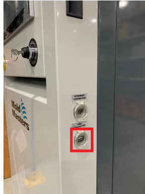
Figure 10-16 USB connections on the side of the controller
