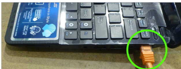
Figure 5-7 Ethernet port on diagnostic computer
