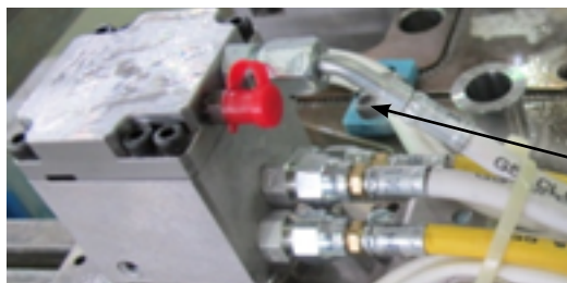
White "G1 Open" hoses go to the lower ports
