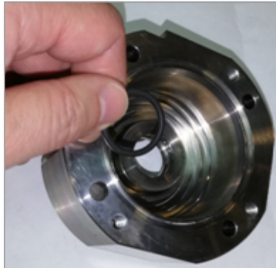
Figure 4-13 Install O-ring for rod seal
